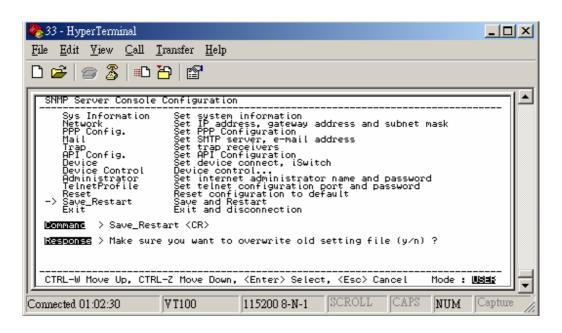
19. Once you have finished with the entire configuration, cursor down to Save\_Restart and hit enter. Make sure you want to overwrite the old settings (y/n)? Hit the y key, then hit enter.
